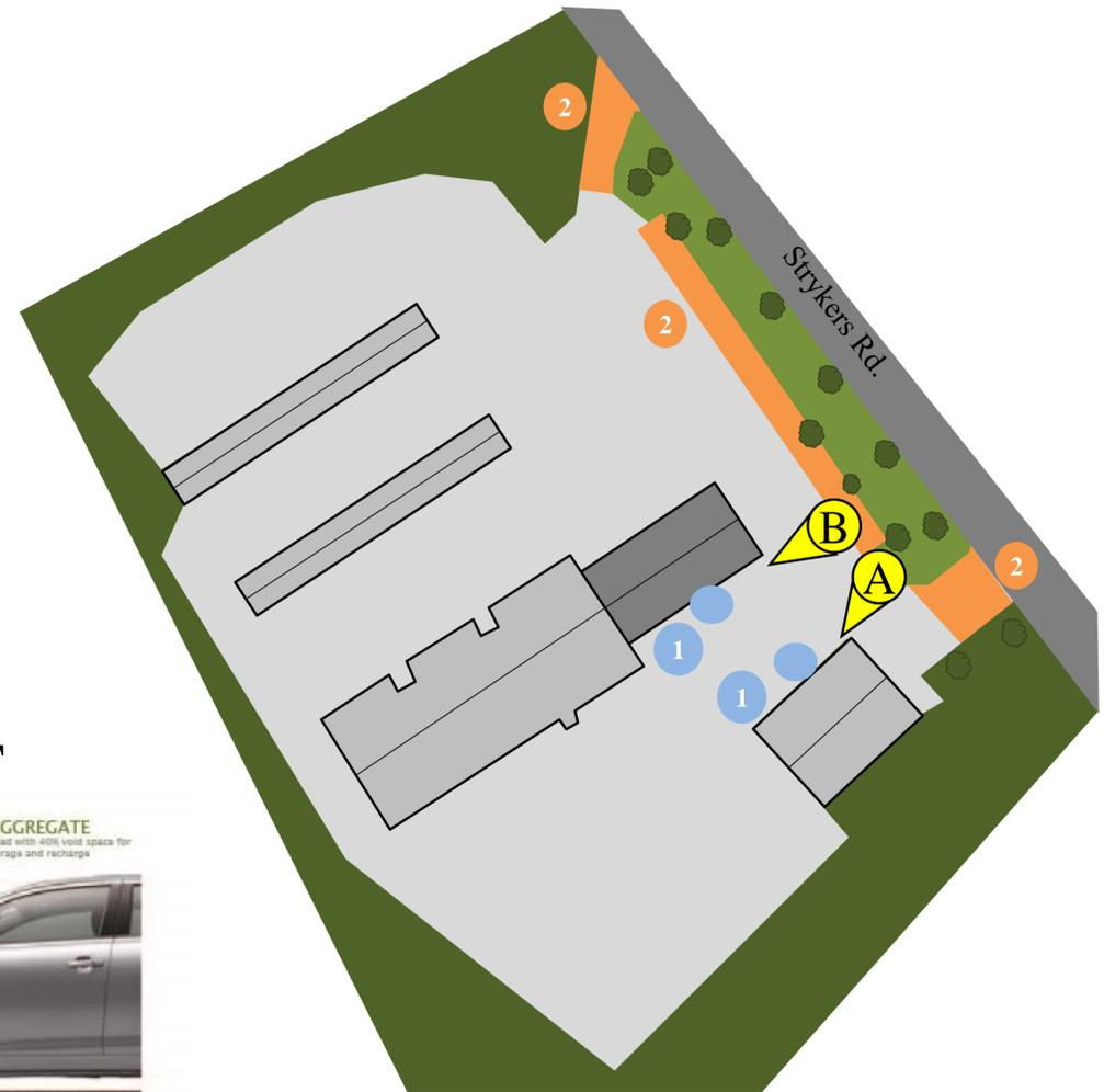
**1 RAINWATER HARVESTING SYSTEM:** Cisterns could help capture the stormwater that drains from the building's rooftop. Connecting the downspouts to the cisterns would allow the stormwater to be collected and used for washing trucks.
