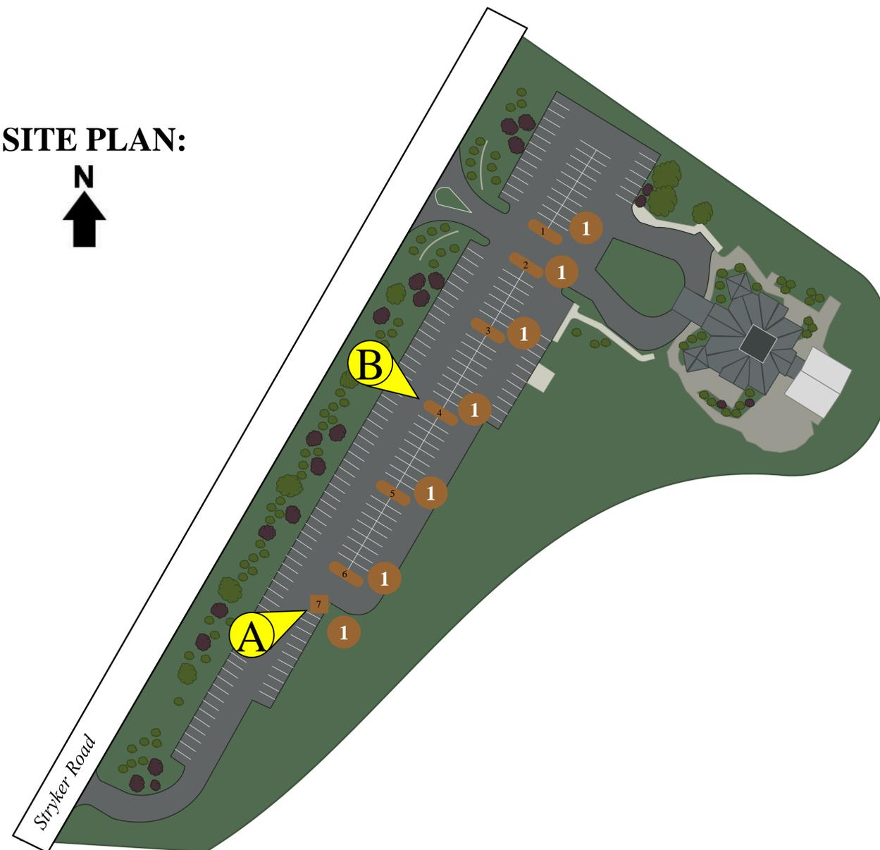
**1 TREE FILTER BOX:** The islands that are currently located in the parking lot could be converted to tree filter boxes. These tree boxes could capture, treat, and infiltrate runoff from the parking lot. Any excess runoff would be conveyed to the existing catch basins through an overflow bypass system. The tree boxes could reduce sediment and nutrient loading to the local waterway while accentuating the property's beautiful landscaping.
